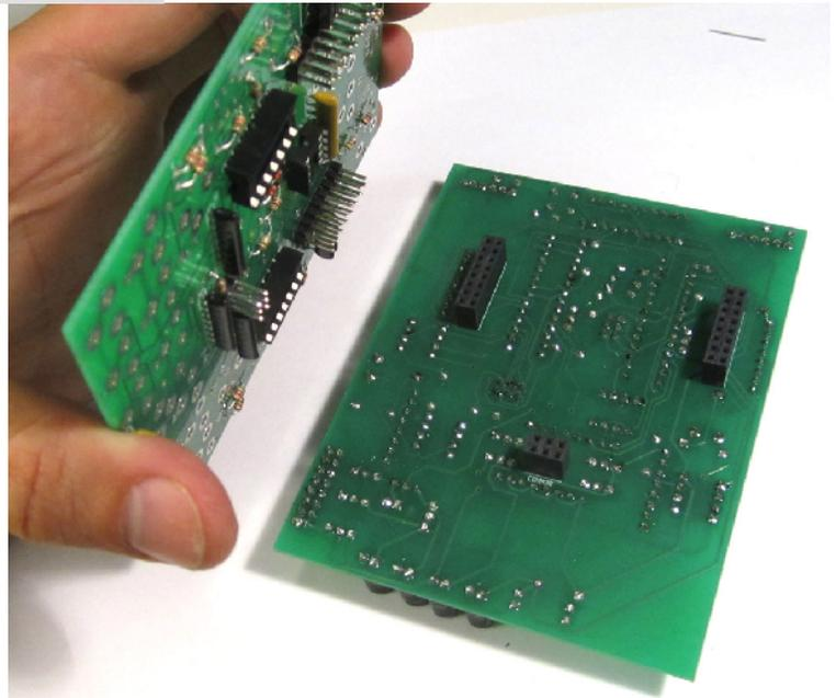
D. Gently press the boards together. Verify that everything is straight and none of the headers are at an angle, and no pins are sticking out.
