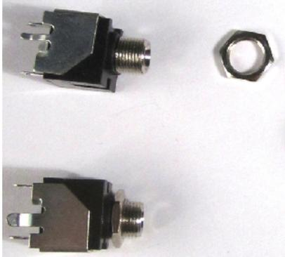
A. Put a hex nut on each of the 22 jacks. Finger tighten the nut (don't use a wrench). Insert the 22 jacks into the PCB. Do not solder yet.
