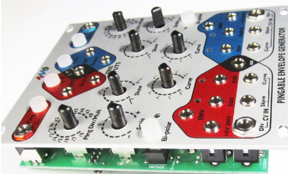
A. Push the LEDs down close to the PCB. Take the panel and gently lower it down on the PCB. Wiggle it slightly so that it fits over the pot shafts, then the buttons, then the jacks.
