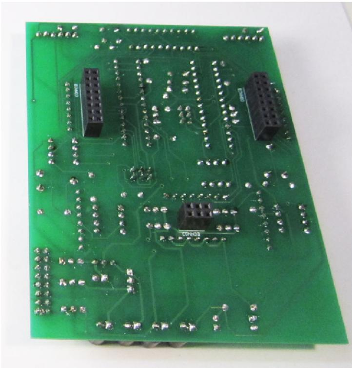
B. Flip the smaller board over so the resistors, sockets, etc are facing down. Insert the 3 female headers as shown. **Do not solder yet!**
