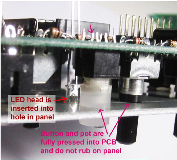
A. Hold the unit so the panel is facing the floor. Gently guide the LEDs by their leads so their heads fit flush into their holes in the panel. You may want to slightly splay their leads out so they stay in place.
