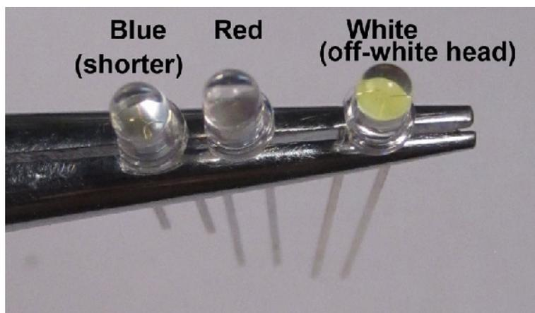
E. Look closely at the 6 LEDs. The ones with short leads are Blue, the ones with milky off-white heads are White, and the clear, long ones are Red. Insert the LEDs into the PCB where marked. The longer lead goes in the square hole.
