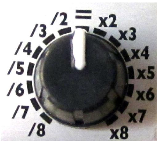
C. Flip the unit over and install the 8 knobs on the pots. Notice how the pot shafts have a D shape, as well as the inside of the knob. Place a spacer under the knob, perhaps a toothpick or a piece of cardboard, so as you push the knob firmly down the shaft, it won't go all the way to the panel and rub when you turn the knob. **The knobs are very difficult to remove, so go slow and be careful.**
