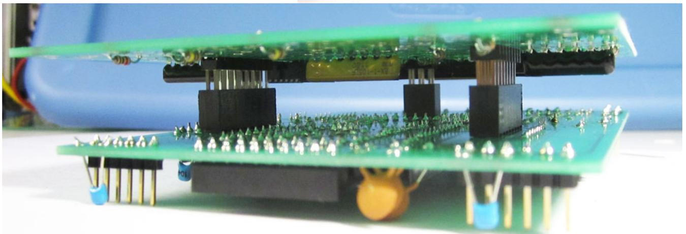
F. Now, squeezing the boards together so the female headers don't fall out, flip the boards over and solder the female headers
