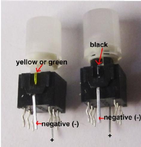
C. Look closely at the six buttons. Four are marked with a yellow mark and two are marked with black. See the photo on left. The side with the black or yellow mark is the negative side. On the PCB, this side is marked with a minus sign (-) as well as the name of the color that should go in that hole. *Note: Green and Yellow are considered the same color.* Insert the buttons into the PCB, being careful that they go in the right way and that no pins are bent.
