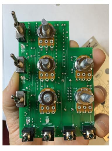
C. Place the 5 pots in the spots as marked on the PCB. Make sure to match the value marked on the pot to the value marked on the PCB. Place a washer on each pot.
