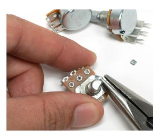
B. Mount the 10-turn pot to the panel with the orientation as shown. Tighten the nut on the top side of the faceplate by hand (finger-tight). You may need to adjust the pot slightly in a later step.
