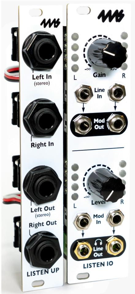
The Listen IO version 1.1 and later versions have four headers: LINE IN and MOD OUT on the top; MOD IN and LINE OUT on the bottom. You can use two of these pairs with a single Listen Up module. (If you have two Listen Up's then you can use all four headers).
