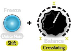
**Crossfading** controls what happens when an oscillator's pitch before quantization falls between two notes of the scale. To understand this feature, you must first understand how the oscillators and scales work. See [Scales and Oscillators](#) section and diagram (pages 11 to 13).
