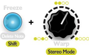
There are two output jacks, **Out A**, and **Out B**. If you patch into **Out A** and leave **Out B** unpatched, then all oscillators will be routed to **Out A**. However, if you patch into both jacks, the oscillators will be panned between the two jacks. The **Stereo Mode** feature controls the panning. Hold the **Shift (Freeze)** button and turn the **Stereo Mode (Warp)** knob to adjust this feature. There are three **Stereo Mode** settings.
