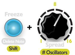
The **Ensemble Oscillator** can potentially use 16 oscillators to produce sound. By default, the module uses all 16 available oscillators, but you can reduce the number of oscillators with this feature.
