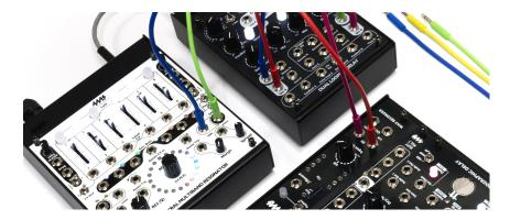
4ms Pods are low-cost, portable, compact enclosures that turn Eurorack modules into table-top instruments. Pods come with an integrated power supply which allows you to daisy-chain multiple units in different configurations using only a single power brick.
