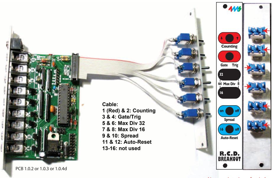
Note oreintation of switches (missing pin is on the left or right side)
