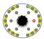
If you purchased your **SWN** and a printed copy of this addendum was included in the box, then you have version 2.x already installed. If you need to double-check, watch the light ring when you power on the **SWN**. Version 2.x has a red light at the 3:00 position in the inner ring, and a blue light at the 12:30 position on the outer ring (see diagram at left).
