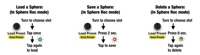
If you accidentally delete a Sphere, you can restore it by moving the flashing light to the empty Sphere slot and pressing and holding **Fine** + **Preset** for six seconds. If the light flashes multi-color rapidly, then a deleted Sphere has been found. Un-delete the Sphere by releasing **Fine** and **Preset** and then tapping **Preset**. If you save over a deleted Sphere, or if you power the SWN off, the Sphere cannot be un-deleted.
