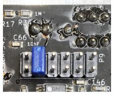
The DLD can operate with full 24-bit audio by installing a jumper on the back of the module in the position 2 as shown in the photo. You can use the BUSCLK jumper if you're not using BUSCLK, or you can use any 0.1" spaced jumper shunt.
