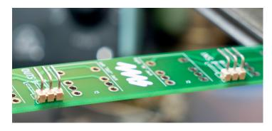
headers are flush with the board. If not, reheat the center pins and adjust. You can use your fingers to adjust if you're careful not to touch the hot pin, or you can use needle-nose pliers to be safer. Once the headers are in correctly, solder the remaining pins.
